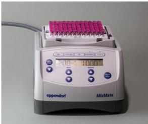
An Eppendorf MixMate plate shaker, a compact white device with a digital display and several control buttons. It is shown with a pink 96-well microplate resting on its top surface. |
