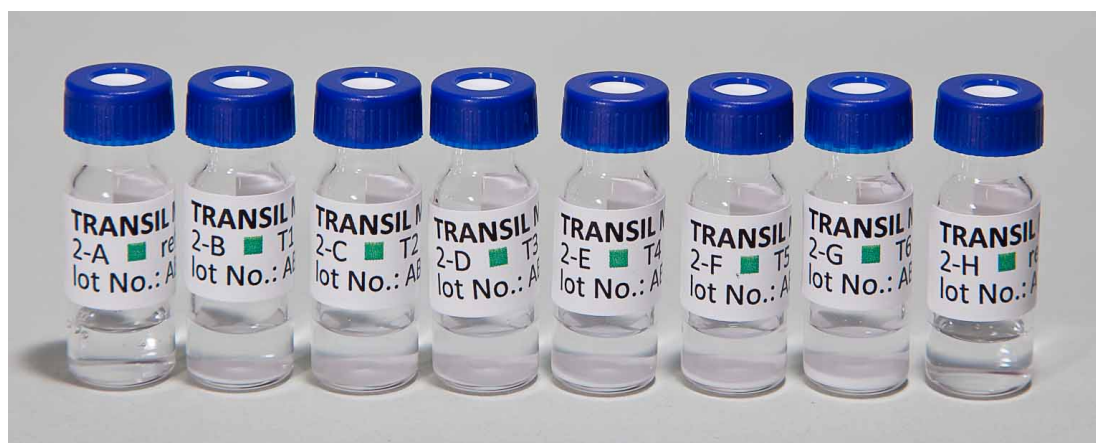
Figure 1: Photograph of vials supplied with the TRANSIL Membrane Affinity kit. The assay uses 8 vials to determine the affinity of drug candidates to membranes.
