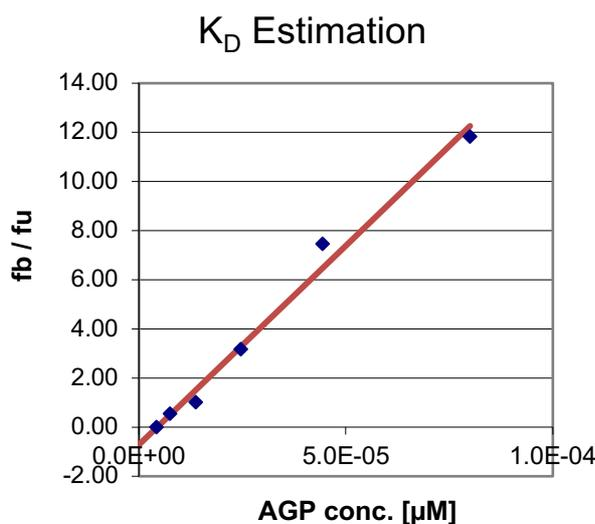
Figure 5: Illustration of fitting experimental data to equation (3) to determine the affinity to AGP. The intercept was estimated to  $-0.7$ , hence a quality score of 5 was attributed to the model fit.
